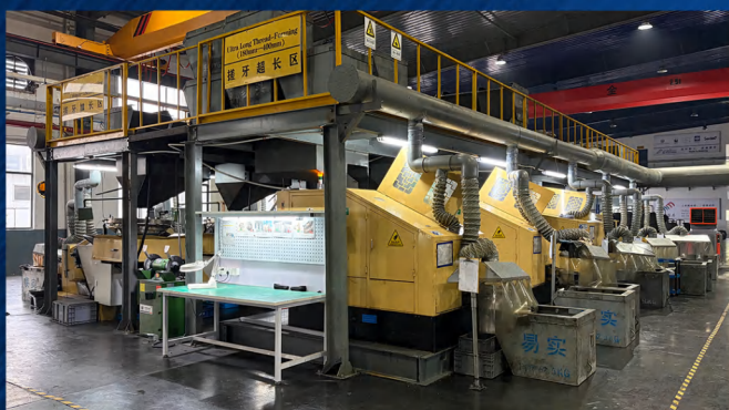
Ultra Long Thread Forming (100mm-400mm)
